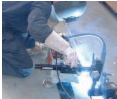
Above: Gullco KATBAK with self-adhesive tape fits through cut outs in the strong backs. The use of KATBAK in this application enabled single sided welding (below) on the outside of the sphere...resulting in the root side of the joint inside the sphere (right) being as good as the outside.
