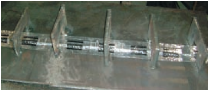
Above: Gullco KATBAK with self-adhesive tape fits through cut outs in the strong backs. The use of KATBAK in this application enabled single sided welding (below) on the outside of the sphere...resulting in the root side of the joint inside the sphere (right) being as good as the outside.
