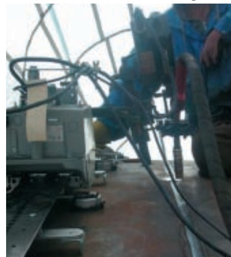
Above: Gullco Flex Kat Oscillator Combination runs on Gullco flexible track held in position using magnetic mounting assemblies
