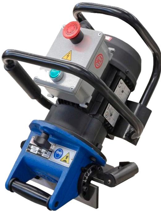
60mm (2.36 in) diameter milling cutters with nine inserts
