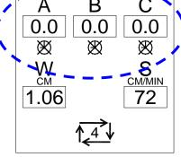
the Technical Manual, GD-098-T for details). The current value is displayed on the LCD screen. Width adjustments can be changed at any time before or during operation and will take effect on the next travel past the B location. Note:- there is a width range where the oscillation stroke is too small to permit A, B & C dwells to work.
