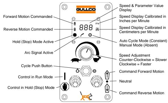
The control has an L.E.D. display that indicates the travel speed in either inches per minute or centimetres per minute. The display also shows the travel direction accessed as well as the status of the Stop command.
