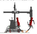
Dual gun holder assembly mounted on the MOGGY® enables positioning of two guns and simultaneous activation of two wire feed signals. MOGGY® is guided by the workpiece.
