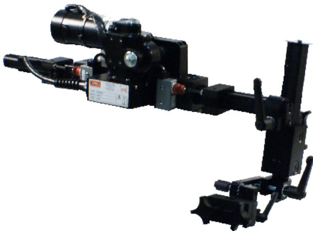
The Gullco remote controlled indexing system is typically used to automate orbital overlay welding or surfacing applications. After each activation of the rotation limit switch the motorized arm will travel a preset distance, in a preset direction at a variably controlled speed (indexing) to produce the desired weld pattern. Variations on the process parameters are available to the operator through the easy to use programmable control.
