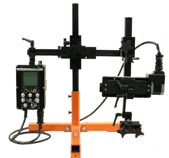
The remote control oscillator is ideal for use with a manipulator stand (KR-1000-WSB) and excels in pipe welding applications in combination with a weld positioner. \*support stand and bracketry sold separately
