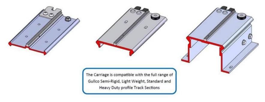
The difference between the Semi-Rigid and the Light Weight track, is the fact that the rack is cut into small sections on the Semi Rigid to allow it to flex better.
