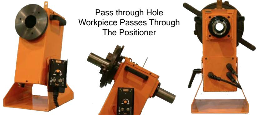
Pass through Hole Workpiece Passes Through The Positioner
