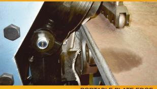
PORTABLE PLATE EDGE **BEVELLING MACHINE**
