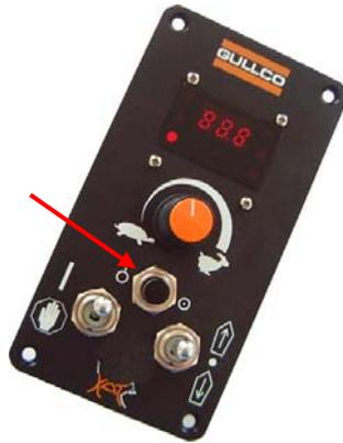
The Cycle Push Button is used to enter the programmable parameters menu that allows the operator to change their values and settings and so define how the automatic cycle will function. The Cycle Push Button is located between and above the Run/Stop switch and the Forward/Neutral/Reverse switch of the GSP control.
