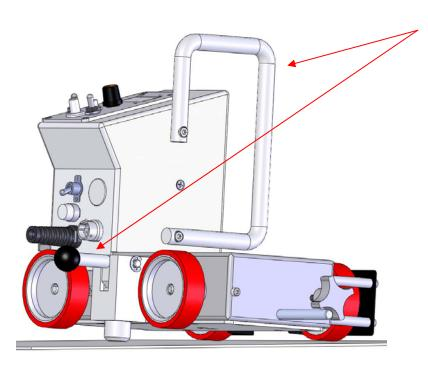
WITH THE RELEASE LEVER LOCKED IN THE DOWN POSITION, LIFT THE MOGGY CARRIAGE BY THE HANDLE
