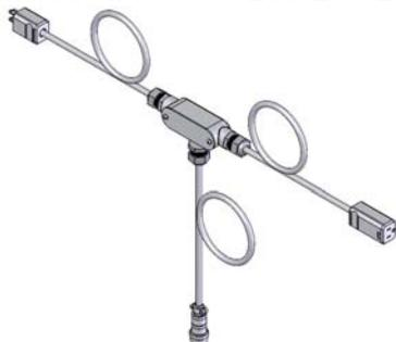
**PENDANT EXTENSION CABLE:** Extension Assembly provides an additional 15ft of length to the Remote Pendant P/N PK-200-368. The maximum combined total length of Remote Pendant cable and Extension cable must not exceed 50ft. Distances over 50ft will result in communication signal loss between the Main Control and Remote Pendant causing erratic operation of the PIPE KAT® system.
