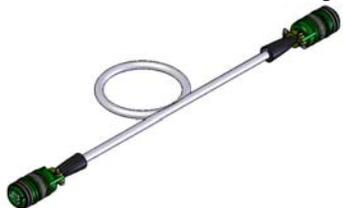
**CARRIAGE UMBILICAL EXTENSION ASSEMBLY:** Extension Assembly provides an additional 25ft of length to the carriage umbilical assembly P/N PK-500-163-G/N/W. The maximum combined total length of Carriage Umbilical assembly and Extension assembly must not exceed 50ft. Distances over 50ft will result in communication signal loss between the Main Control and Carriage causing erratic operation of the PIPE KAT<sup>®</sup> system.
