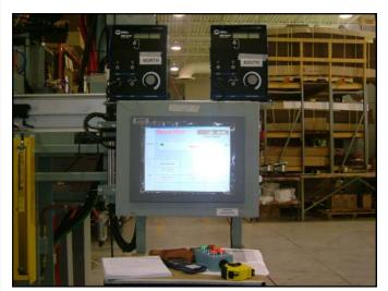
Touch screen industrial PC utilizing Citect HMI software.
