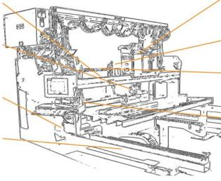
X-AXIS TRAVERSE CARRIAGE powered by Gullco KAT® 24volt gear motors.
