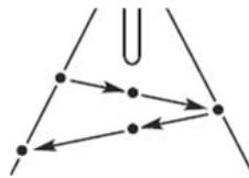
The proper torch angle/position is established quickly and easily with the Gullco KAT® Oscillator Head. It's simply a matter of tilting the oscillator, which can be adjusted side to side or forward and backward this results in the elimination of the time consuming and generally ineffective procedure of tilting the carriage or track.
