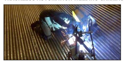
The Magnetic MOGGY® is intended to automate and improve the quality of welding and cutting operations by carrying the welding gun or cutting torch, at precisely controlled speeds, along the path of the joint as well as providing the interface between the welding and cutting motion and the arc start and stop signal. The Magnetic MOGGY® is normally guided by adjustable guide wheels which are used to keep a set distance from the joint path.
