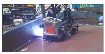
The Magnetic MOGGY® is intended to automate and improve the quality of welding and cutting operations by carrying the welding gun or cutting torch, at precisely controlled speeds, along the path of the joint as well as providing the interface between the welding and cutting motion and the arc start and stop signal. The Magnetic MOGGY® is normally guided by adjustable guide wheels which are used to keep a set distance from the joint path.
