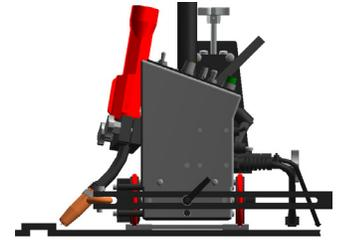
The MOGGY® is performing a lap joint weld. It is guided by Industry Standard 6" (152.4mm) v-groove track running parallel to the joint.
