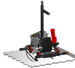
The MOGGY® performing a fillet weld using a template, guide or fence positioned parallel to the workpiece. The actual workpiece is often used as the guide.
