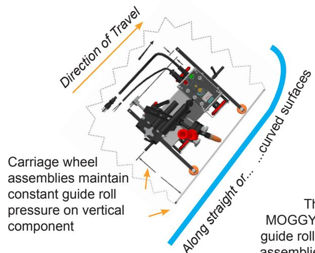
Carriage wheel assemblies maintain constant guide roll pressure on vertical component
