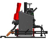
The MOGGY® is performing a lap joint weld. It is guided by Industry Standard 6" (152.4mm) v-groove track running parallel to the joint.
