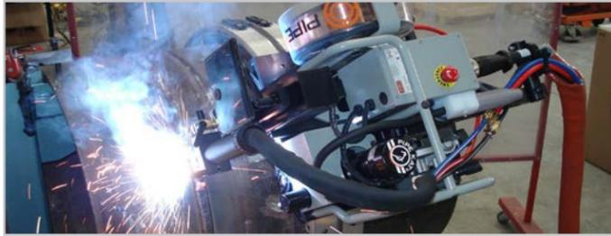
The Pipe KAT® is a pipe welding carriage designed for orbital welding. It is an electrically powered track guided carriage that operates in the forward or reverse directions at precisely controlled speeds. The carriage operates on a track band made of durable aluminum extrusion by engaging the track with self-aligning wheels and a rack and pinion drive. This wheel assembly uses a lever to engage that track making it very quick and simple to install the carriage.
