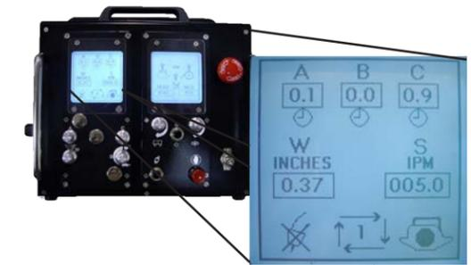
The Remote pendant (left) is used in conjunction with the main control (right) to provide adjustment during setup, initiate the weld cycle, provide fine adjustment during welding, and to stop the weld cycle.
